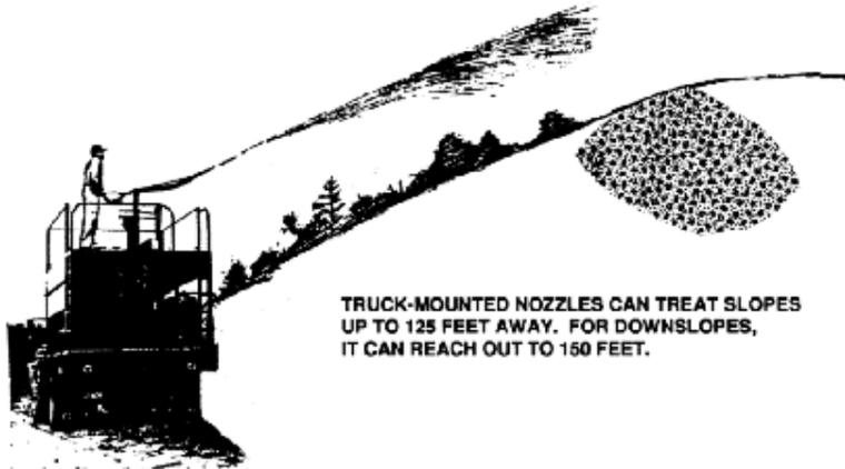
TRUCK-MOUNTED NOZZLES CAN TREAT SLOPES UP TO 125 FEET AWAY. FOR DOWNSLOPES, IT CAN REACH OUT TO 150 FEET.
